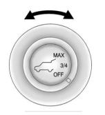
On vehicles with a power liftgate the switch is located on the driver door. The vehicle must be in P (Park) to use the power feature. The taillamps flash when the power liftgate moves. Choose the power liftgate mode by turning the dial on the switch until the indicator lines up with the desired position. Press the center of the switch.
